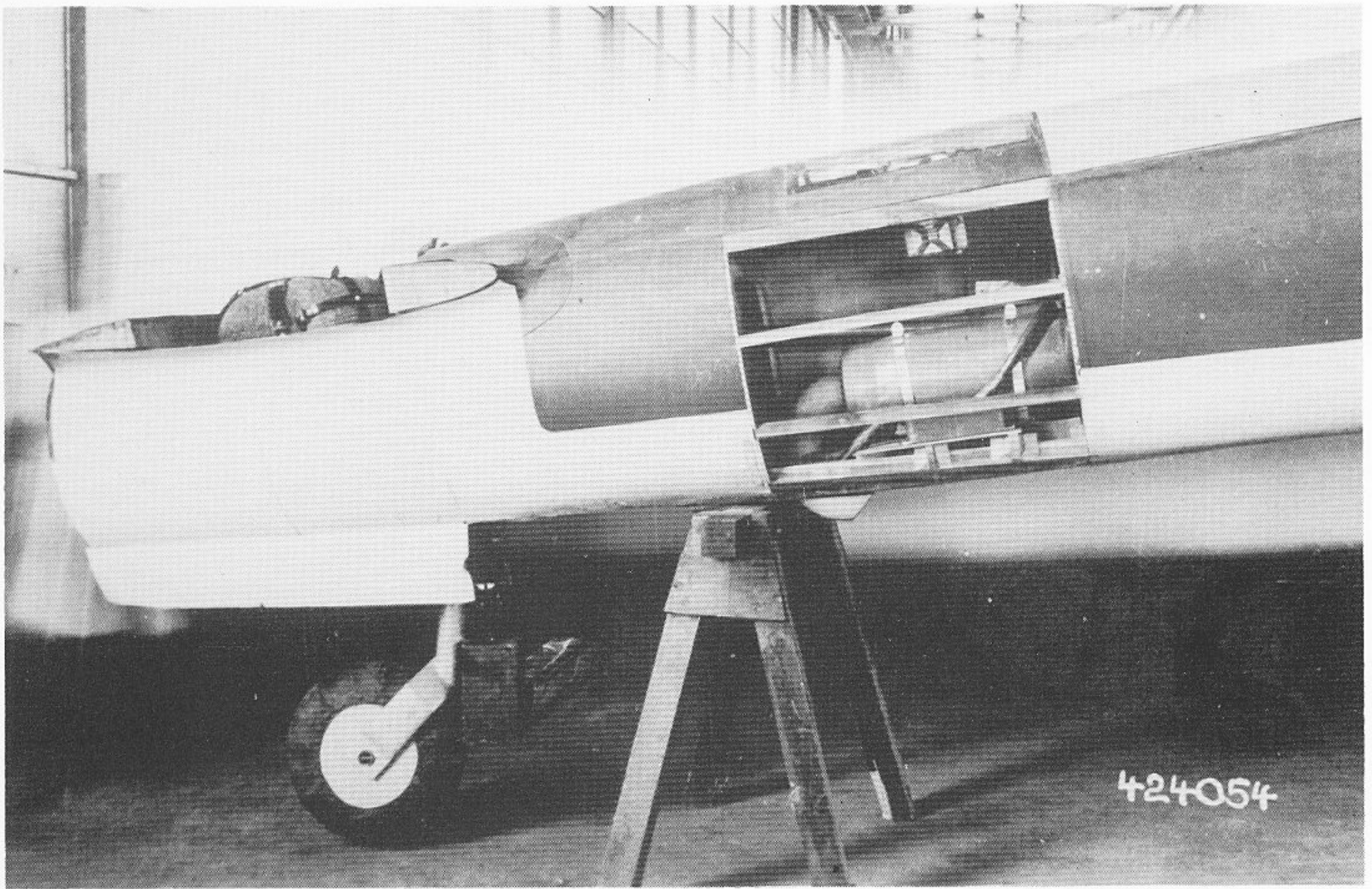
Rear fuselage of the Ar 240 V3. The tail unit has yet to be installed.
